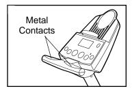
To use the handgrip pulse sensor, place your hands on the metal contacts. Your palms must be on the upper contacts and your fingers must be touching the lower contacts. Avoid moving your hands. When your pulse is detected, the heart-shaped indicator in the display will flash each time your heart beats. After a moment, two dashes (--) will appear and then your heart rate will be shown.
