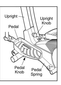
To adjust the upright, first turn the upright knob counterclockwise a few turns to loosen it. Next, pull the knob, raise or lower the upright to the desired height, and then release the knob. Move the upright up and down slightly until the pin on the knob snaps into one of the four adjustment holes in the upright. Make sure that the upright is not resting on top of the pin. Then, turn the knob clockwise until it is tight.
