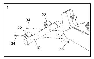
Whilst another person lifts the back of the Frame (1), attach the Rear Stabiliser (9) to the Frame with two M10 x 75mm Carriage Bolts (34) and two M10 Nylon Locknuts (33).
